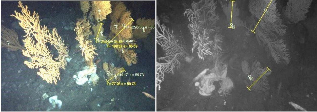
Figure 23. In situ stereo images showing the method for estimating Primnoa pacifica colony sizes using Sebastes 1.3 software (Williams et al. 2016). Euclidean triangulation is used to estimate distance based on the comparison between six measured values in two calibrated cameras mounted on a sled.
