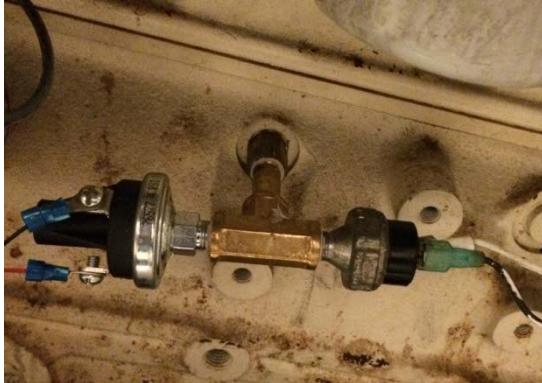
Engine oil pressure sensor installed on vessel engine. Located in the engine room.
