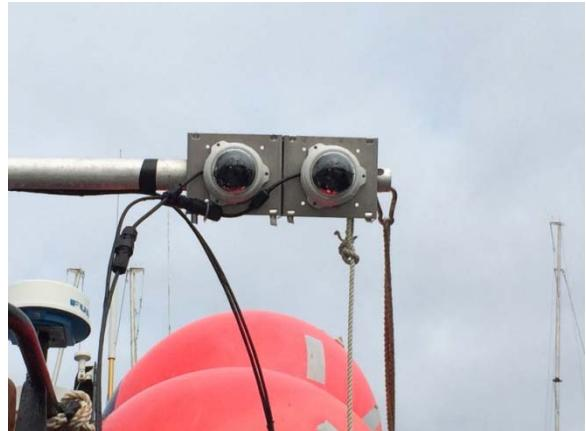
Aimed at the starboard hauling station to provide a close-up to confirm species identification.
