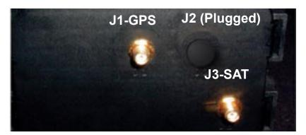
7) Connect the GPS antenna cable to connector GPS (\*\*PT)) a Witt 1 to conn
