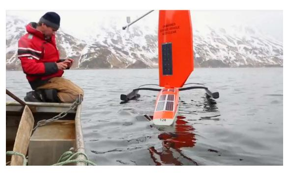
A wind- and solar-powered autonomous sailing vessel controlled from shore through satellite communications
